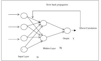
**Notes:** The weight connecting node i in the input layer to node j in the hidden layer is denoted by Wji, and the weight connecting node j to the output node is represented by Vj
